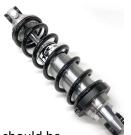
**Step 6.** Retainer should be tight on the shock body with zero movement or play once installed. Your spring and spring retainer installation is now complete.
