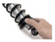
Step 3. With anti-seize applied on your spring retainer threads, set screw installed (hand tight at this point); thread the retainer onto the coilover shock body.
